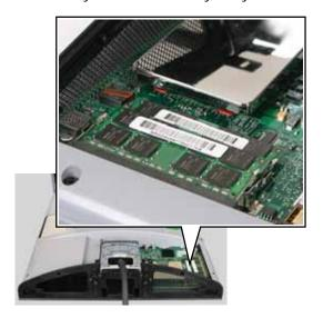
If you are removing an old module from a memory slot, spread the two metal tabs away from the sides of the memory module. The module flips up at a 30° angle. If you are removing a module from the lower memory slot, you must first remove the module from the upper slot.
